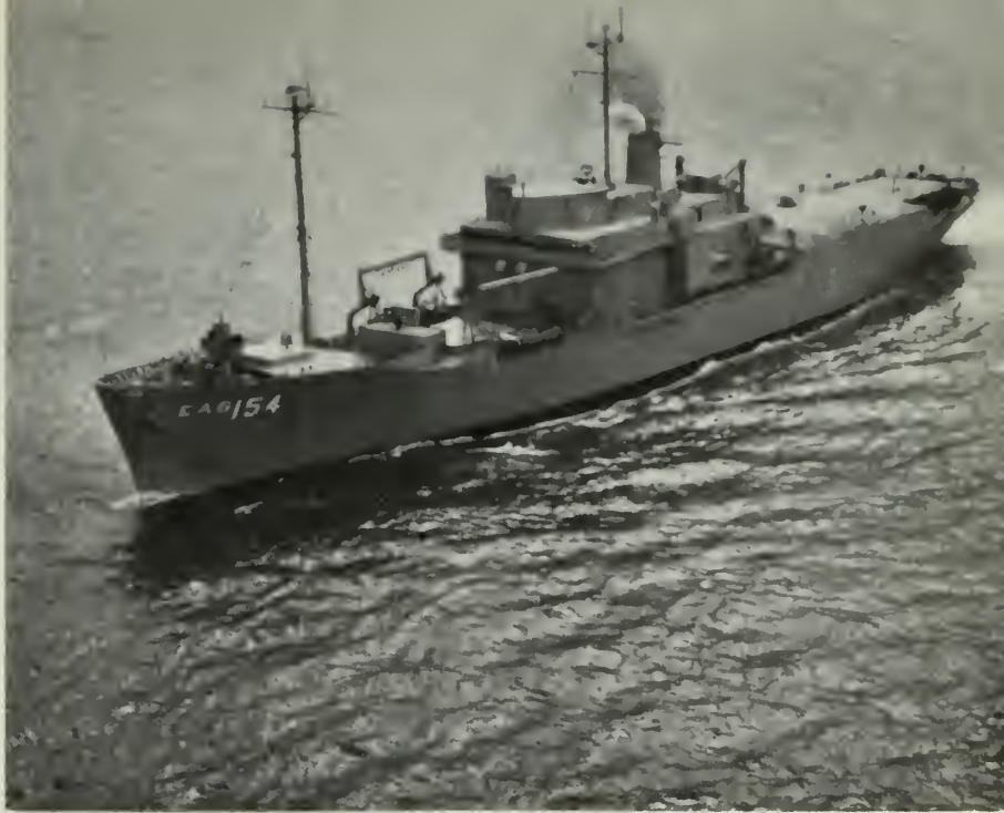
SEAGOING LAB—USS Observation Island (EAG 154) will test launching, fire control and navigational devices required for fleet ballistic missile Polaris .
